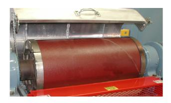
The position of the pressure roll in respect to the cylinder is controlled by micrometer had-wheels graduated in .001". The adjustment is so accurate that print can be sanded from ordinary newspaper without harming the paper itself.
