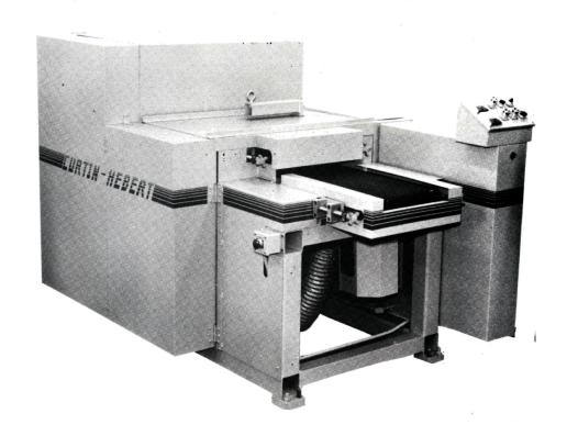
Deburring & Surface Finishing of small magnetizable parts.
