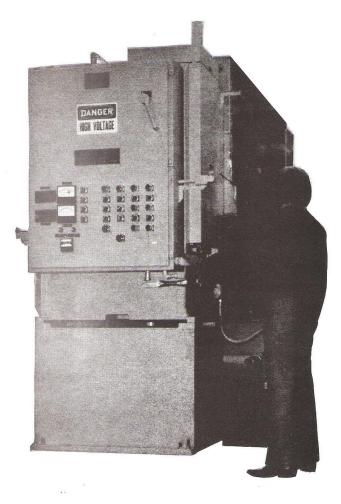
Mechanical surface finishing & cleaning of coil up to 72" wide.
